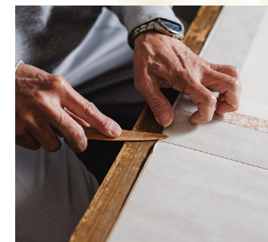
The amount and thickness of the glue varies by the material of the mounting. "The most critical aspect of my work is how I apply the glue," says Mr. Uchida.
