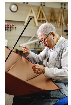
“Middle stitching” is the process of sewing the fabric to the ribs. The umbrella's beautiful silhouette derives from this meticulous work.
