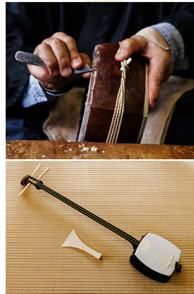
Top: Unlike a violin, a shamisen does not gain value as it ages. Rather, it deteriorates, requiring regular tuning. The ideal sound is achieved by shaving the body and neck and replacing the skin. Bottom: The body is made of wood, such as rosewood or quince. Rosewood can only be sourced through authorized agencies because of Washington Convention restrictions. It is also getting harder to obtain the skin and plectrum materials.
