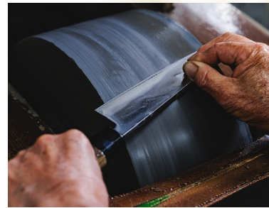
A round whetstone is used for rough grinding. Back when the fish market was in Tsukiji, the whetstone was used so continuously that the blade had to be replaced almost every month.
