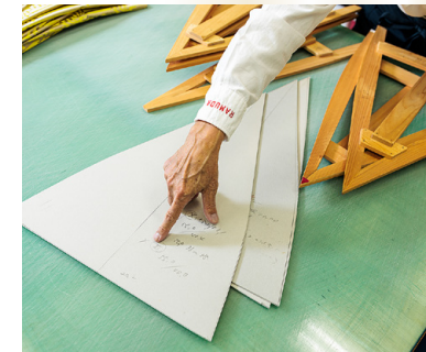
Before making a wood mold, Mr. Hayashi makes many prototypes out of thick cardboard. He writes both the previous and the current measurements on them, so that he can see the process of revision at a glance.
