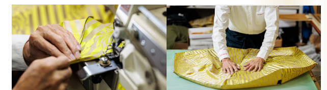
Left: The cut pieces of fabric are sewn together so that the patterns connect. Right: The fabric is sewn together to form a circle, then sewn to the ribs by hand.
